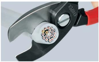
Final cut: after cutting the sheath in the front profile the conductors in the rear part are cut. Initial cut in the front profile, final cut in the rear profile — to keep it as easy as possible.
