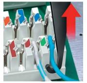
Putting down and cutting the cable in one operation
