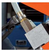
Sealing the hose connection on central lubrication
