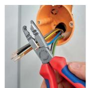
Cutting edges shortening of single wires
