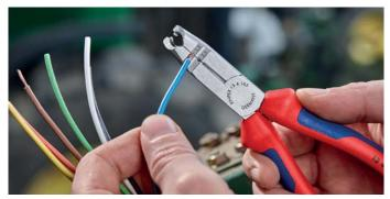
Stripping holes for conductors of 1.5  $\text{mm}^2$  and 2.5  $\text{mm}^2$
