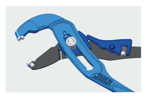
The locking mechanism on the spring hose clamp pliers permit simple and safe work, even with closed clamps. Modern CAD technology simulates the mechanism on the screen.
